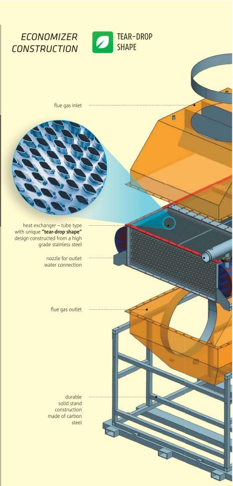
eLINE casing – easily ..... removable metal panels insulated with mineral wool allow for inside surface inspection and cleaning
