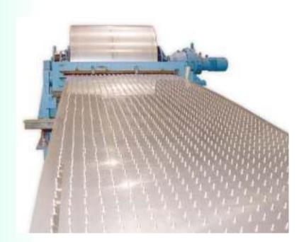
SEC Spiral is an assembly of two long sheets, usually separated by studs, wrapped to form a pair of concentric spiral channels. Alternate edges are closed and seal welded. Covers on each side complete the Spiral. Connections are installed on the "shell" and covers to provide true counter-current flow.
